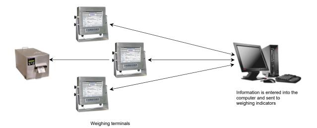
Weighings performed on each terminal are automatically transferred to the host computer as and when they are made, and the labels are printed. It is thus possible to monitor the real-time production from the main computer.
